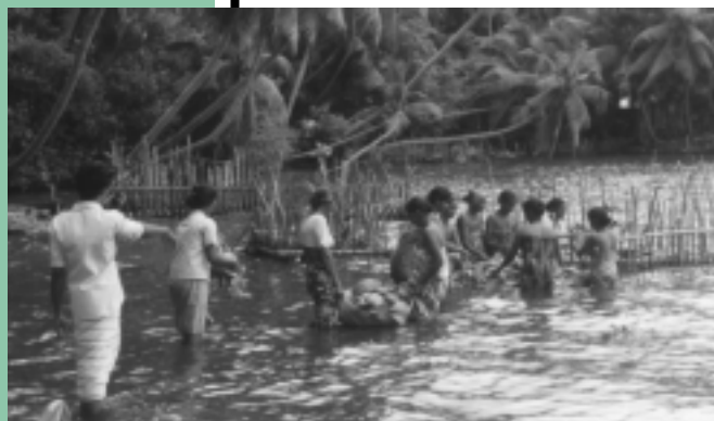
Husks soaking for coir yarn production
